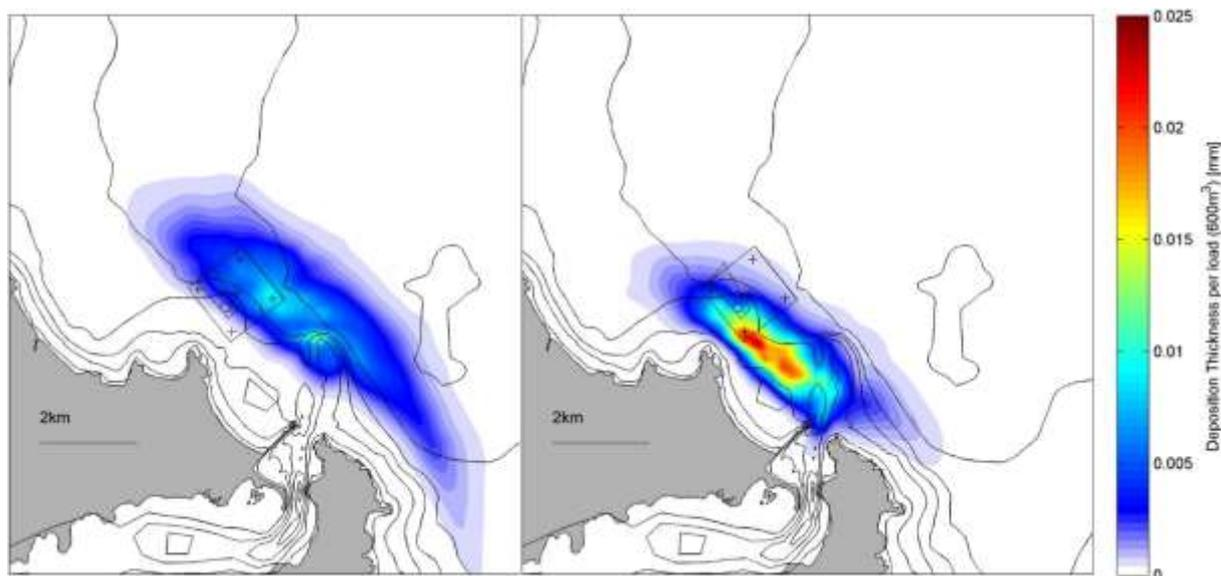
**Figure 3-2: Suspended sediment (passive plume only) settlement contours 12 hours after release (c. 2 m depth) of 600 m<sup>3</sup> of silty dredgeate from dredge New Era at each of two points (left, site 2, greatest dispersion; right, site 3, least dispersion) within the proposed enlarged Heyward Point dredged sediment placement ground. Note, deposition scale differs from that in Figure 3-3. Hydrodynamic conditions averaged over a full year. Courtesy of MetOcean Solutions Ltd.**
