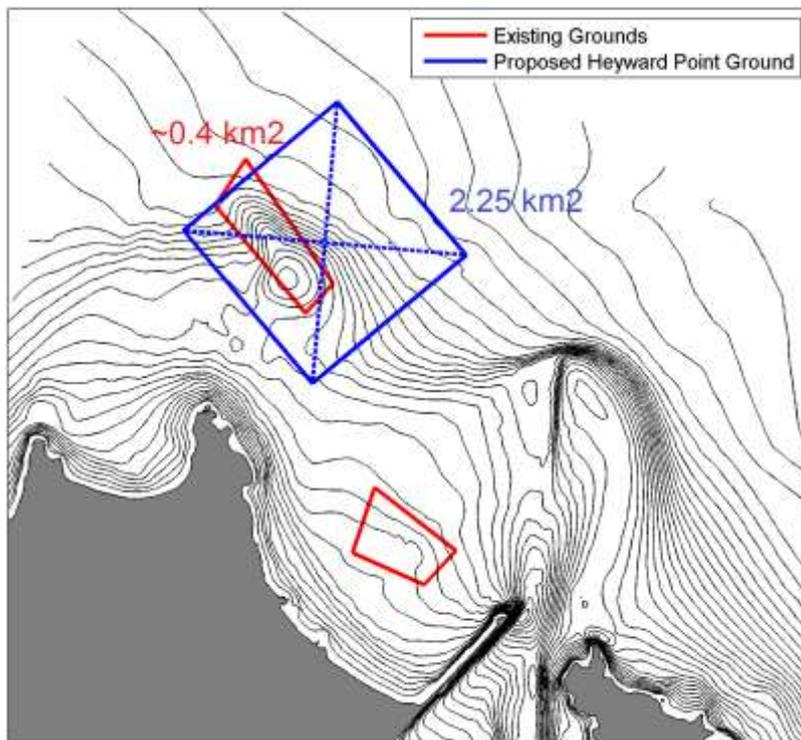
**Figure 4-1: Existing dredged sediment disposal grounds (red rhomboids) and proposed enlarged ground (blue square) incorporating the existing Heyward Point ground.** Courtesy of Port Otago Ltd.
