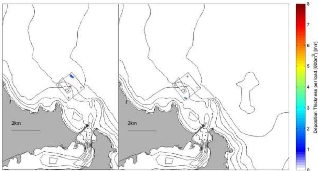
**Figure 3-1: Suspended sediment (passive plume only) settlement contours 12 hours after release (c. 2 m depth) of 600 m<sup>3</sup> of fine sand dredgeate from dredge New Era at each of two points (left, site 1, greatest dispersion; right, site 3, least dispersion) within the proposed enlarged Heyward Point dredged sediment placement ground. Hydrodynamic conditions averaged over a full year. Courtesy of MetOcean Solutions Ltd.**
