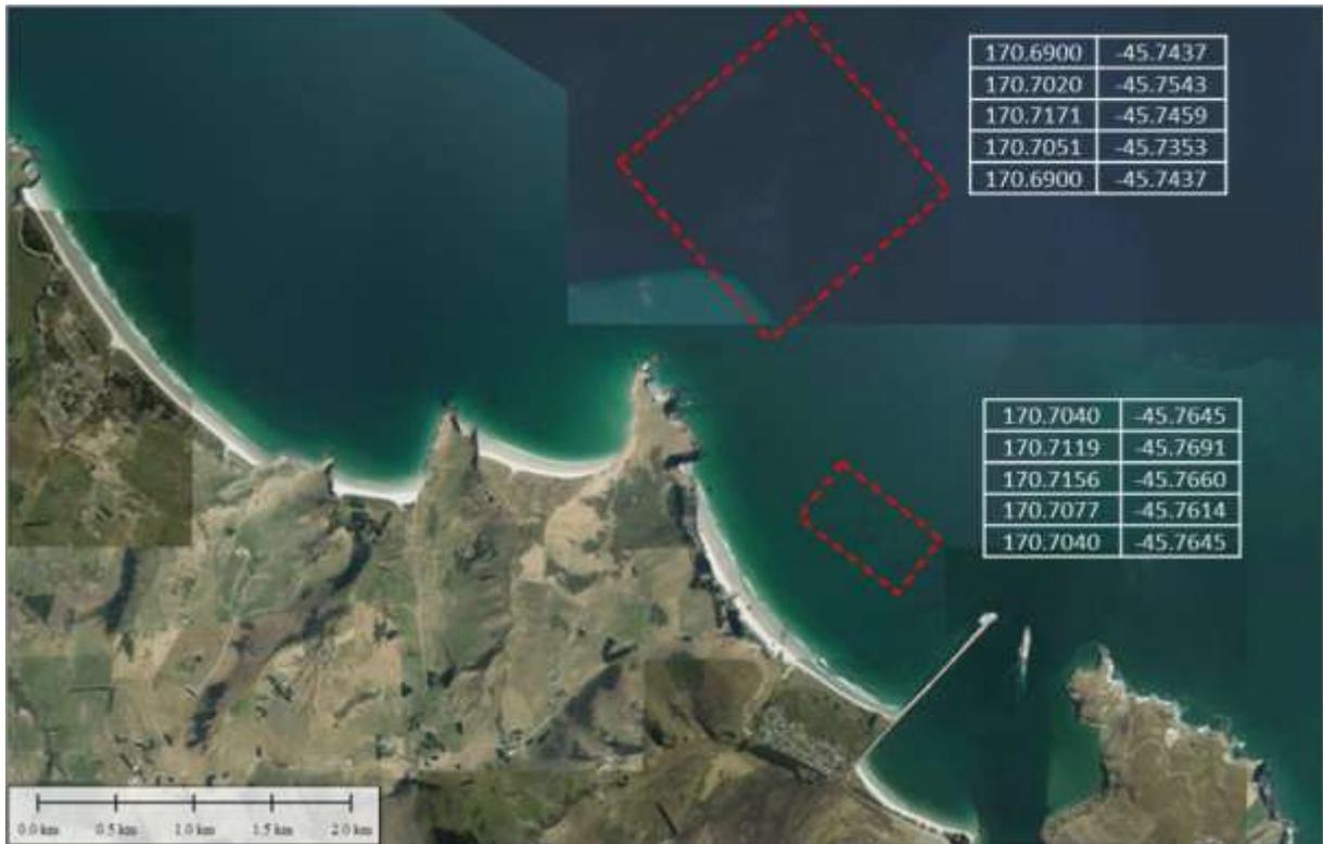
**Figure 1-3: Proposed enlarged dredgeate placement grounds for maintenance dredging sediments off Heyward Point and Aramoana. From: MetOcean (2016).**
