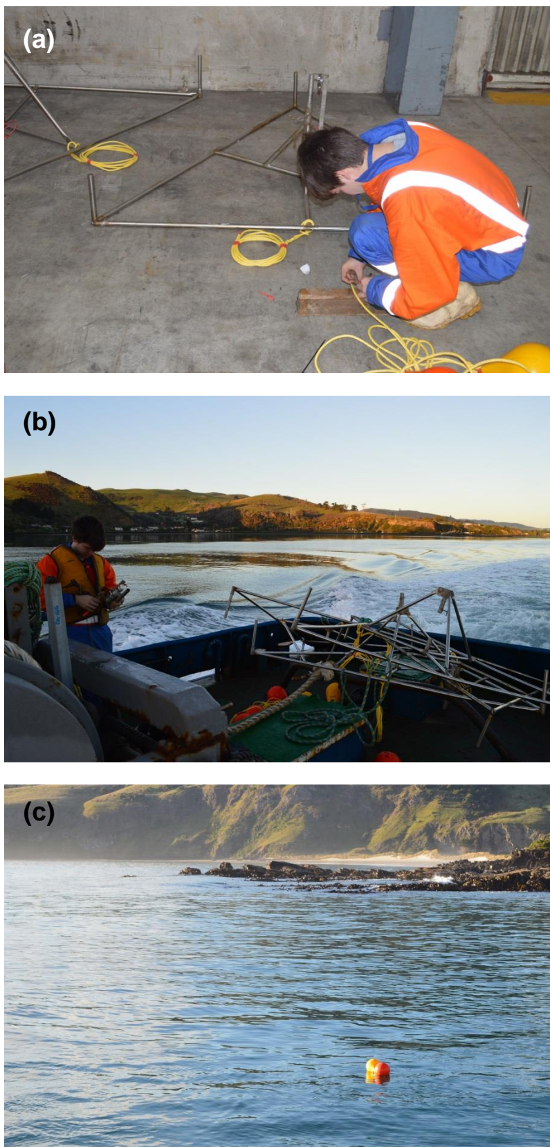
Figure 2.10. RBR deployment at site W1: (a) triangular frame where the RBR was installed; (b) overview of the deck of boat used in the second day showing the RBR; (c) marker buoys deployed with the RBR frame.
