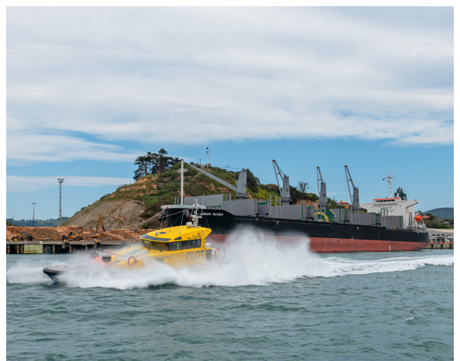
Te Rauone is powered by a Volvo D16 750 horsepower engine with two 17" Deon water jets. She is capable of top speeds up to 30 knots, is self-righting and able to handle all weather conditions.
