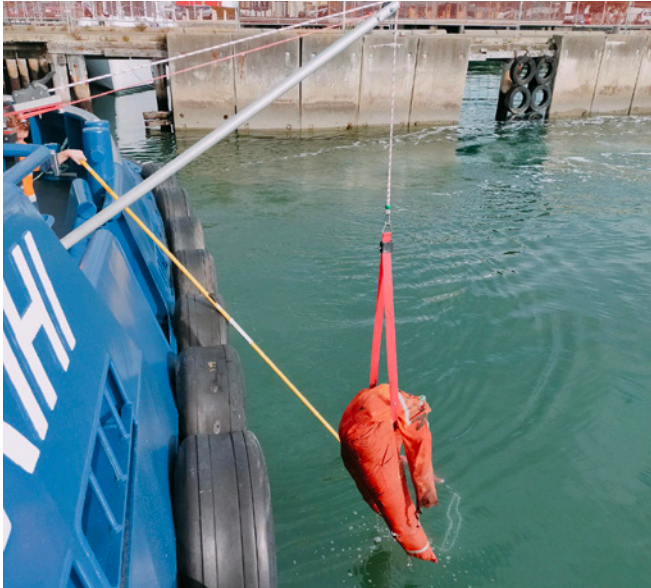
The tug Arihi recently had a new “person overboard” system installed and the crew gave it a big tick. During their first training session, they averaged less than six minutes for retrieval, in line with international benchmarks.
